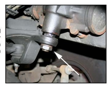
The 1-1/4" Deep socket (180 lbs-ft) should be used to install the new sector shaft nut, re-using the stock lock washer.
