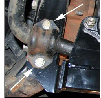
Tighten the four sway bar mounting bolts (17mm) to 40 lbs-ft (as per Dodge Specification).
