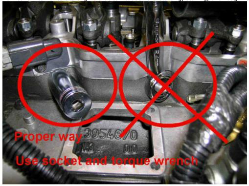
Tighten the injector hold down bolts alternately to 89 inch pounds. Then tighten the connector tube to 37 foot pounds. Tighten the injector wire connector nuts to 11 inch pounds. Be very careful to not over tighten.
