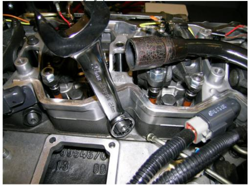
Using Miller 9015 connector tube puller, thread the tool into the connector tube and pry/pull the tube straight out. The nut is still in place in the photo, but obviously needs to be removed first. If you don't have the 9015, you really risk damaging the connector tube threads if the tube sticks in the head.
