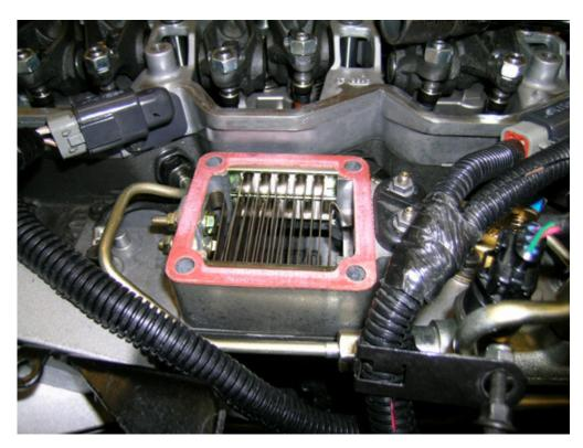
Remove 10mm bolts on plastic valve cover, cover. Remove hoses from breather box.
