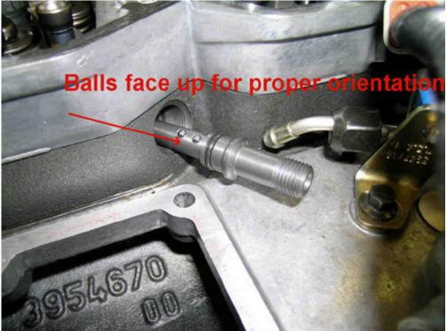
Tighten the connector tube to 11 foot pounds. This is the step most technicians' short cut by using a box end wrench to tighten the connector tube. By not correctly installing the tube, you risk leaks internal to the engine that can cause hard starting, stalling, and rough running etc.
