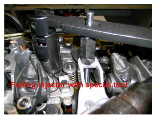
If you do not have the special tool, be very careful as you pry the injector out by prying on each side of the hold down a little at a time
