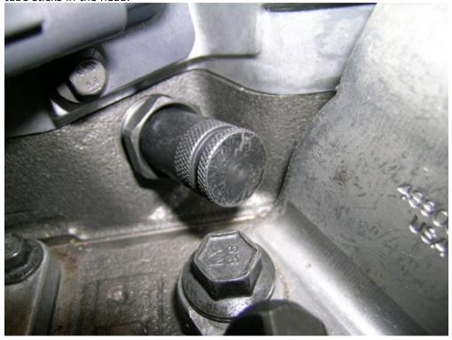
Remove 10mm bolts holding exhaust rocker arms, these are in the middle of the rocker, and sometimes covered in oil. Make sure to keep track of which cylinder these came from. Remove 8mm injector wires. Remove 8mm injector hold down bolts.
