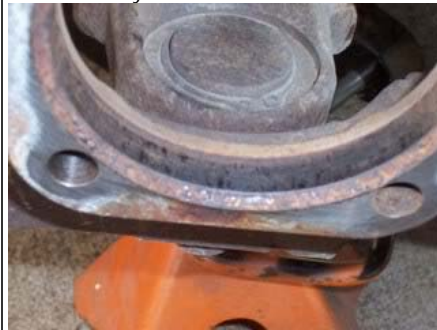
After removing the nuts on the ball joint the outer will fall off and you can just chain it and the tie rod out of the way. If you need to use a pickle fork leave one nut on some, if not the thing will jump off and get you. Its heavy.
