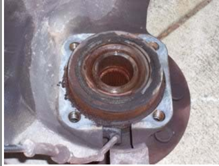
After the bearing has been pulled then you can pull the axle shaft. It shows more rust and also the circle clip on the Ball Joint you need to remember to remove. Now is a good time.
