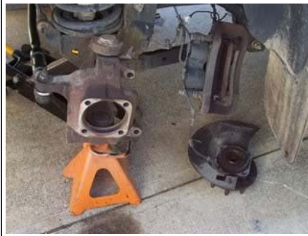
Close up of the bearing and some of the rust.
